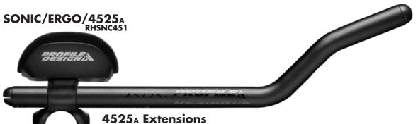
The 4525a extensions have a first section at 45deg and the grip at 25deg. They also have a 7.5mm lateral shift per side (15mm total) to allow fine tuning of the grip width. They are 400mm long to allow a wide range of riders to fit. The cable routing is designed to exit from the rear of the extension.
